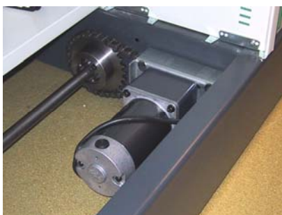
LOGICPlus™ Gearmotor monteret i Bruynzeel M1 mobilreol.
