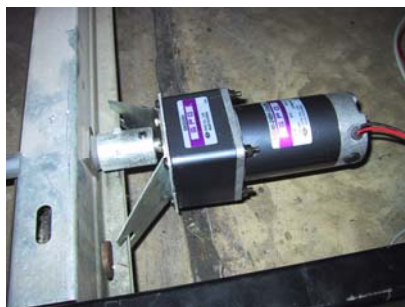
LOGICPlus™ Gearmotor monteret i Electrolux EM80 mobilreol.
